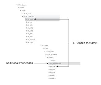
**FIGURE 9-9** Both the USIM and SIM applications can hold ADN records; one EF\_ADN will be duplicated between the USIM and SIM.
