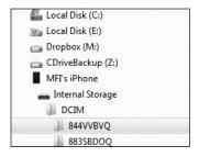
File system view of an iOS device connected as a PTP device—Digital FIGURE 6-1 Camera Image (DCIM) folder is available
