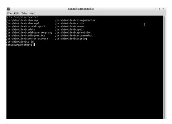
**FIGURE 6-12** Using the Santoku interface to start libimobiledevice to create an iOS backup
