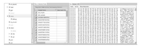
FIGURE 10-1 MMS folder containing some of the additional files unaccounted for in a "tip of the iceberg data" examination
