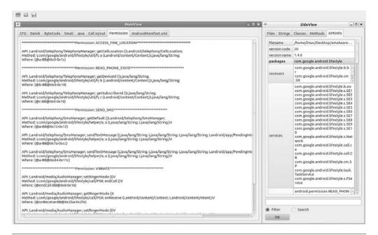
**FIGURE 13-16** APKInspector can be a good static analysis tool that shows permissions, calls, and even code.
