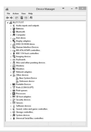
**FIGURE 7-1** If devices are not recognized or the driver cannot be found, they are located in the Other Devices section of the Device Manager.
