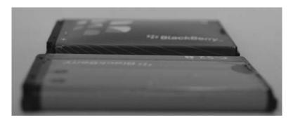
A normal battery (front) and a bloated battery (back). The middle of the back battery is distended and could explode, causing damage to the evidence.
