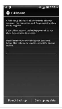
FIGURE 8-9 Screen activated on a connected Android device when running the ADB backup command
