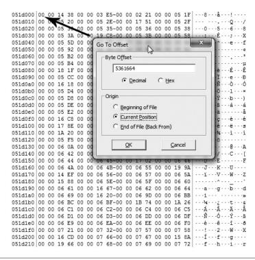
**FIGURE 11-22** The location of the freelist is obtained by using the Go To Offset in FTK Imager.
