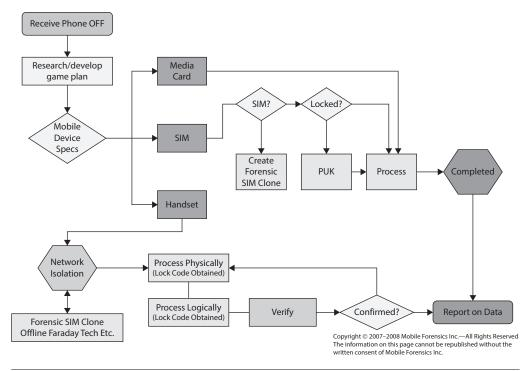
FIGURE 2-2 Processing a mobile device (introduced at Mobile Forensics World 2008)
