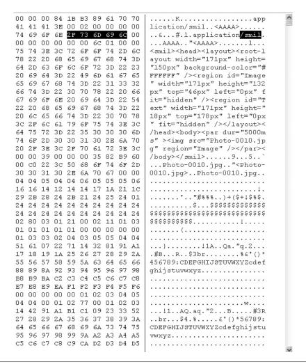
FIGURE 10-6 Using Physical Analyzer to search manually for an MMS message; notice the searched-for string: smil
