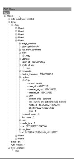
FIGURE 11-37 JSON file from Instagram's fsCachedData folder decoded into a readable format in Notepad ++ with the JSON Viewer plug-in
