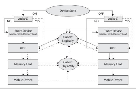
FIGURE 8-5 Mobile device evidence processing workflow
