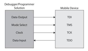
FIGURE 6-8 A simplistic communication model from a software debugger/programmer to and from a mobile device TAP group
