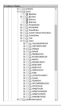
Internal file system of a Windows Phone 8 device displayed in FTK **FIGURE 10-22**
