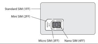
FIGURE 9-1 The evolution of SIM/UICC size
