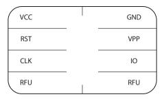
UICC smart card contact points: communication to the chip occurs via the I/O contact, which is the pathway to the UICC CPU.
