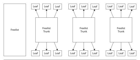
**FIGURE 11-20** The freelist is an index to trunk files that point to leaves where the data is stored.
