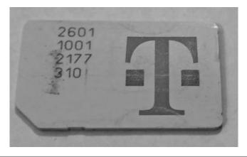
FIGURE 9-5 UICC exterior with a visible ICCID
