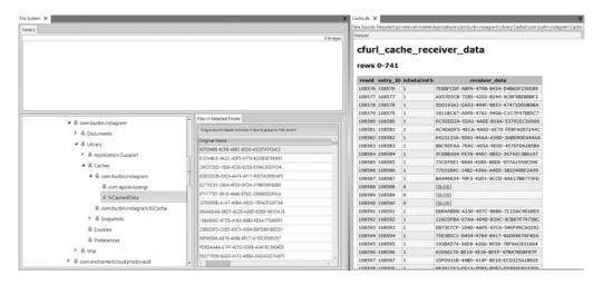
**FIGURE 11-10** The fsCachedData folder in Instagram gives the investigator a folder full of GUID named files that can be matched to the GUID within the cfurl\_cache\_receiver\_ data table.
