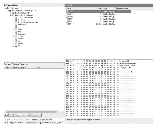
FIGURE 11-3 An iPhone raw disk image with unencrypted unallocated space containing many deleted files
