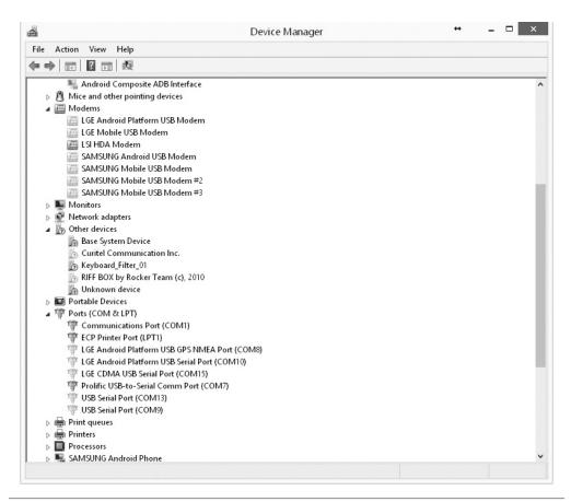
**FIGURE 7-4** Several devices are shown as phantom devices under Modems, Ports, and Kindle (for example, Android Composite ADB Interface, Samsung Mobile USB Modem, LGE Mobile USB Modem).
