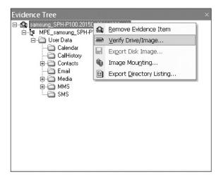
**FIGURE 5-6** Using AccessData FTK Imager, import the created image, right-click the device, and select Verify Drive/Image.
