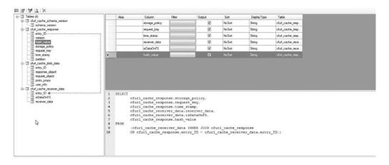
**FIGURE 12-5** A complex query between two tables with multiple rows using a foreign key can be completed in a short time using automated query builders such as SQLQuery Builder.
