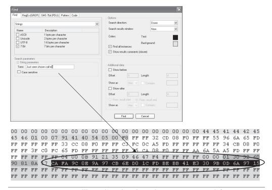
FIGURE 10-8 Using Cellbrite Physical Analyzer, the examiner can search for a string in several formats.
