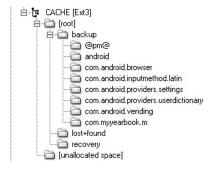
**FIGURE 13-2** The cache partition should be examined for possible evidence when this partition exists within the Android device.
