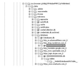
FIGURE 10-21 Navigation into the file system to uncover SQLite databases within the sys.browser application subfolders
