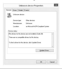
**FIGURE 7-2** The Properties dialog for a device in the Device Manager details the device and associated drivers.
