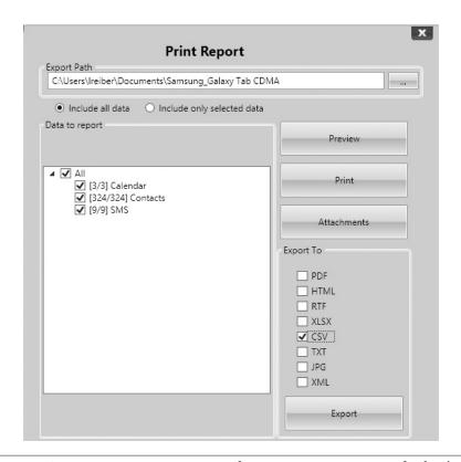
FIGURE 5-1 AccessData MPE+ 5.0 exports data into a comma-separated value (.csv) file.
