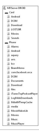
File system view of an Android device connected as a MTP device—notice FIGURE 6-2 the internal and external file systems containing various files and folders
