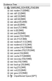
FIGURE 13-1 A JTAG binary file, when imported into FTK Imager, will show as a logical file system under the root folder.
