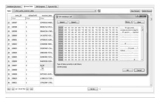
**FIGURE 12-3** Looking into the table cfurl\_cache\_receiver\_data, the examiner can click any record labeled BLOB and the data will be exposed in a separate window, as shown with a video file that can be exported and viewed within a native viewer.
