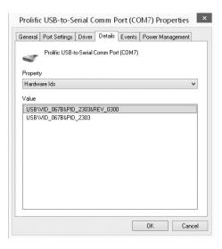
**FIGURE 7-3** The Prolific Cable Properties table under the Details tab identifies the assigned PID and VID for the device.
