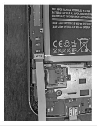
FIGURE 6-11 Molex connector attached to a Samsung S3 JTAG TAP
